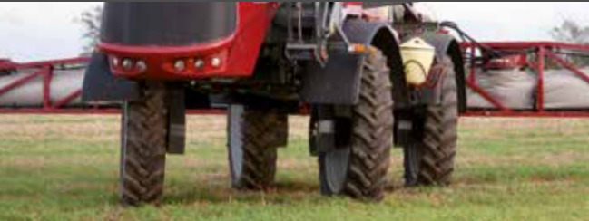
Crab steering – in difficult conditions and manoeuvring
