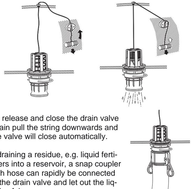
To release and close the drain valve again pull the string downwards and the valve will close automatically.
