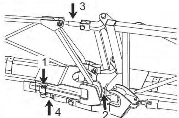
**Adjustment of inner section folding (OLH)**
