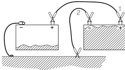
This to avoid sparks near the battery when connecting the last cable to terminal.
