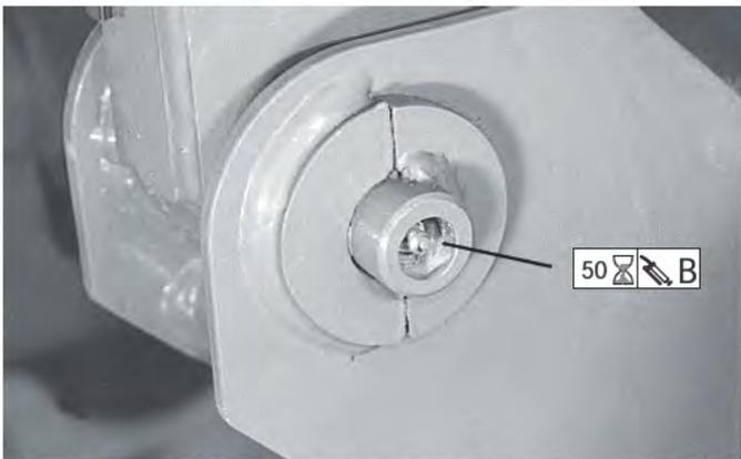
Front/rear axle suspension bearings
