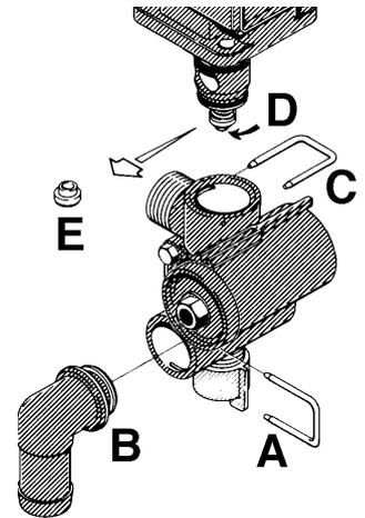
Remove the clip C and lift the EC-motor housing off the valve housing. Then unscrew the screw D and replace the valve cone E. Re-assemble in opposite sequence.
