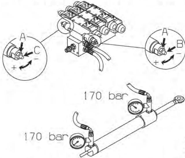
1. Fit two 250 bar pressure gauges at the outer section folding ram.
