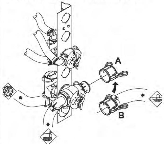
1. Remove cover **A**, and connect suction hose **B** to Suction Manifold.
