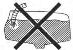
If the hose is lead to the bottom of the tank and the water pump at the water supply plant stops, chemicals can be siphoned back and contaminate water supply lines and well.
