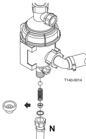
If the required working pressure cannot be obtained, the restrictor is too large. Choose a smaller restrictor. Start with a black one, then a white and finally a red one.
