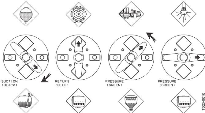
**B.** Rinsing the pump, operating unit, spray lines, etc. in case you stop spraying before main tank is empty (e.g. beginning rain etc.).
