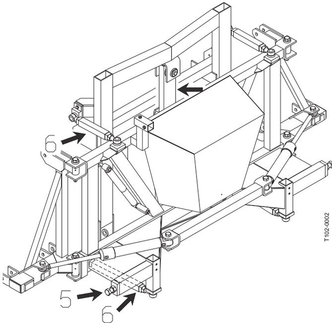
**Adjustment of pendulum suspension (OLH)**
