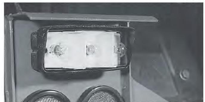
**Front position lamp and direction indicator bulb**
