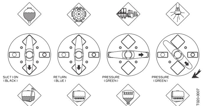
12. When the spray liquid is well mixed, turn handle on the Pressure Manifold towards "Spraying" position. Keep P.T.O. engaged so the spray liquid is continuously agitated until it has been sprayed on the crop.
