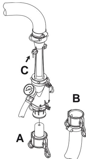
3. Turn handle on Pressure Manifold towards Fast Filler. With the engine at 2200 r/min, the pressure gauge should indicate about 10 bar.
