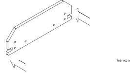
This plate needs to be welded to two longitudinal bearers, which subsequently can be bolted to each side of the tractor.
