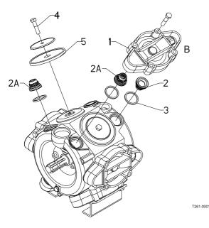
Diaphragm pump overhaul kit (valves, seals, diaphragms etc.)
