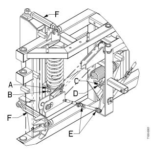
Pendulum return spring and cables
