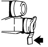
Remove the protection box of the solenoid valves at the boom. The boom can now be operated by pressing the individual buttons on the solenoid valves.
