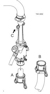
NOTE: Turn handle towards EC-operating unit before turning away from Fast Filler in order to avoid peak pressure blowing the safety valve!
