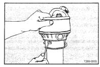
2. Remove the nylon bearing and pull off the protection tube.
