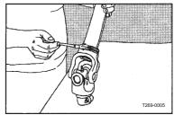
4. Slide on the shield tube and fit the bearings tabs into the slots.
