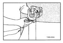
3. Grease protection tube bearing groove on the inner yoke.
