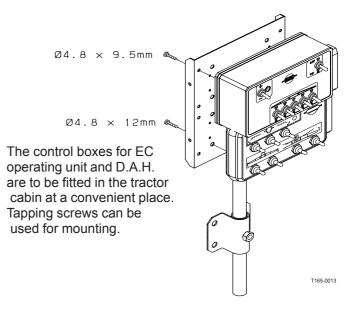
The wires must have a cross-sectional area of at least 4.0 mm2 (#10 awg) to ensure sufficient power supply. The boxes must be fused according to the table.
