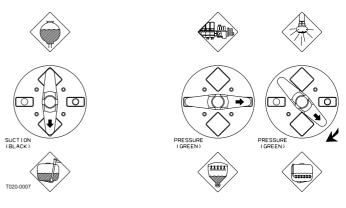
13.When the spray liquid is well mixed, turn handle on the Pressure Manifold towards "Spraying" position. Keep P.T.O. engaged so the spray liquid is continuously agitated until it has been sprayed on the crop.
