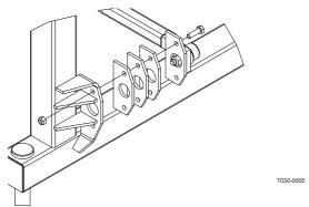
If the boom should follow the movements or inclinations of the trailer the guide rods should be inclined towards each other at the rear.
