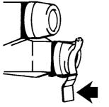
Remove the protection box of the solenoid valves at the boom. The boom can now be operated by pressing the individual buttons on the solenoid valves.
