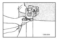
3. Grease protection tube bearing groove on the inner yoke.
