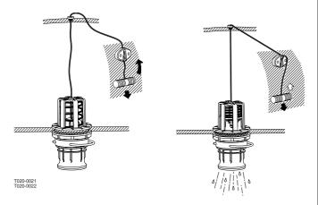
To release and close the drain valve again pull the string downwards and the valve will close automatically.
