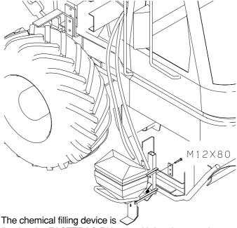
fitted at the FASTTRAC RH step with brackets as shown.
