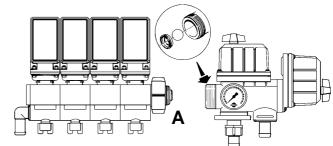
Remove the 2 bolts fixing the main ON/OFF-pressure valve unit to the bracket, unscrew the union nut **A** and pull the valve away from the distribution valves.
