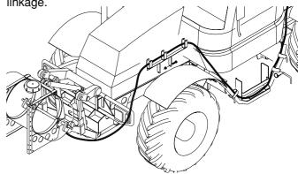
Then fix the hose support on the bracket of the front axle spring suspension on the left side and place the hose. Fix the support in such a way that the longer part is pointed backwards.
