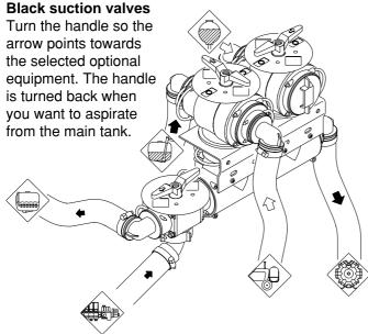
If 2 valves are fitted, eg. Front Tank and Rinsing Tank, select optional extra and turn the other valve to "O" (closed). To resume aspiration from the main tank, the arrow must point towards the main tank. Remaining valve must be closed.
