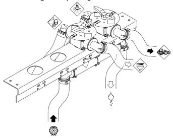
If 2 or more valves are fitted, the arrow must point towards the optional extra you select. Remaining handles are turned to "O" (closed). When spraying is to resume, select the Self-Cleaning Filter/operating unit. The other handles are turned to "O".
