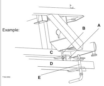
**IMPORTANT!** Each fitting must be mounted to the spray boom right between two triplets. Failure to do so may disturb the spray pattern during the application of pesticides.
