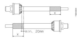
**NOTE!** The shaft must always have an overlap of minimum 155 mm (6.1 in).
