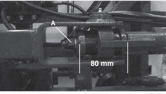
**IMPORTANT!** Each set of rubber dampers on both of the cylinders must be equally tightened. Therefore, control that the distance between the two plates, shown on the picture, is **80 mm** on both cylinders.
