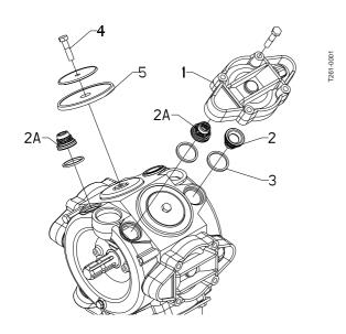
Diaphragm pump overhaul kits (valves, seals, diaphragms etc.)
