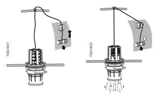
To release, pull the string downward and the valve will close automatically.
