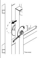
2. Turning the eccentric axle clockwise will decrease the gap between the wheel and the lift. Use a spanner.
