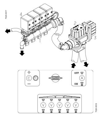
Before spraying, the EC operating unit is adjusted using clean water (without chemicals).
