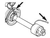
8. To ensure long life of the transmission shaft, try to avoid working angles greater than 15°.
