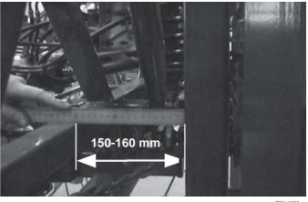
3. When correct setting has been obtained, tighten nuts A on the turnbuckle again.
