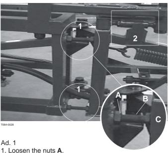
2. Screw the bolts B a bit inwards to create some space between the boltheads and the profile C.
