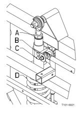
Anticlockwise rotation: The spring arrangement becomes shorter and the steering arms are moved upwards
