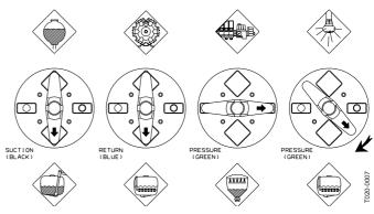
13.When the spray liquid is well mixed, turn handle on the Pressure Manifold towards "Spraying" position. Keep P.T.O. engaged so the spray liquid is continuously agitated until it has been sprayed on the crop.
