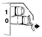
If the tractor is equipped with closed centr hydraulics, e.g. John Deere, button (O) must be pressed in.
