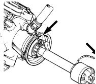
To ensure long life of the P.T.O. shaft, try and avoid working angles greater than  $15^{\circ}$ .
