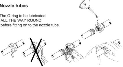
In case of leaks: DO NOT overtighten, disassemble, clean and reassemble as shown.
