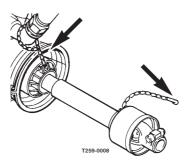
8. To ensure long life of the transmission shaft, try to avoid working angles greater than  $15^{\circ}$ .
