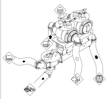
Turn the handle so the arrow points towards the selected optional equipment. The handle is turned back when you want to aspirate from the main tank.
