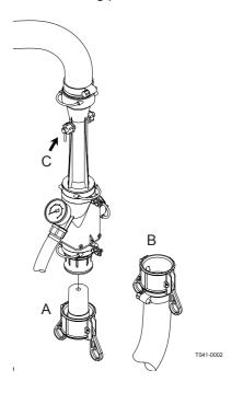
**NOTE!** Turn handle towards operating unit **before** turning away from Fast Filler in order to avoid peak pressure blowing the safety valve!
