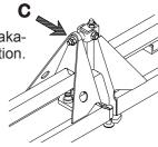
3. Parallel adjustment of outer section
