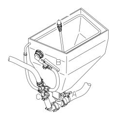
**NOTE!** The scale in the hopper can only be used if the sprayer is parked at level ground! It is recommended to use a measuring jug for best accuracy.
