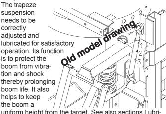
uniform height from the target. See also sections Lubrication and Re-adjustment of the boom.
