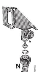
When cleaning the filter remove hose  ${\bf N}$  and the hose at the safety valve and check there are no residues.
