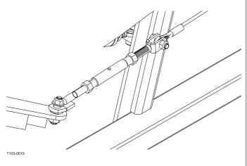
If 18-21 m boom: Turn the turnbuckle another 4 complete turns and retighten the jam nuts.
