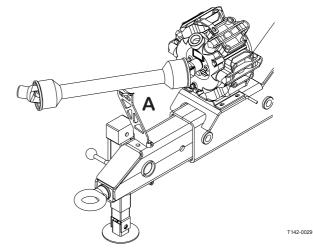
At High hitch models the transmission shaft is placed in the hook underneath the drawbar when not in use.
