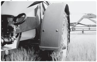
Mudguards can be fitted on the trailer wheels by means of a supporting frame which is bolted to a mounting on the wheel axle.
