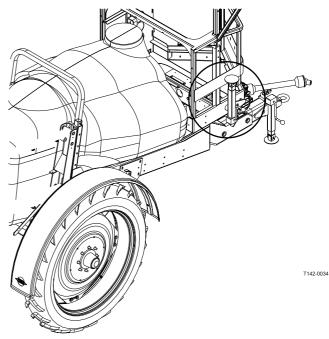
To remove the support leg: Lift the leg, remove the linch pin and pull out the support leg.
