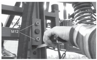
Measure and adjust the jaw if necessary by means of the two M12 bolts .
