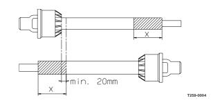
**NOTE!** The shaft must always have a minimum overlap. The size of this overlap depends on the pump model:
