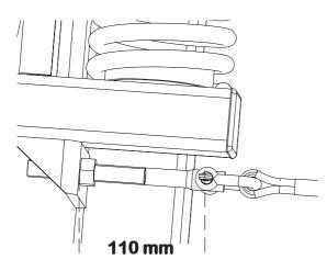
Properly adjusted cables will be very tight and only deflect a small amount (mm) when pulled by hand.
