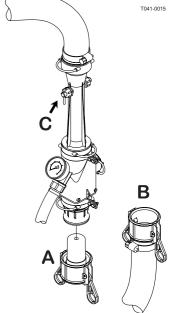
**NOTE!** Turn handle towards -operating unit **before** turning away from Fast Filler in order to avoid peak pressure blowing the safety valve!
