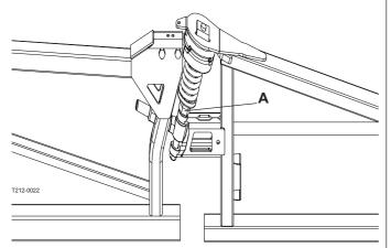
SPC type breakaway is shown here. Same principle applies for SPB type.
