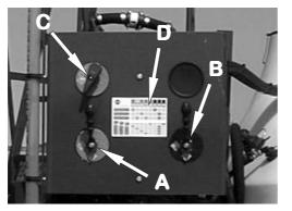
On the Agitation/Rinsing valve a function is activated/opened by turning the handle towards the desired function Closed
