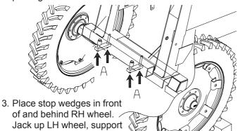
4. Loosen clamp bolts for LH wheel axle.
