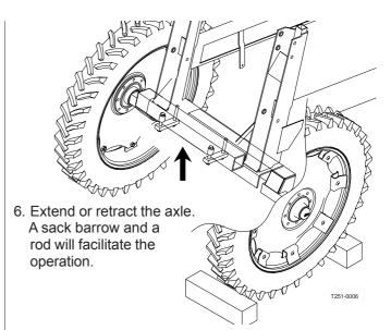
7. If the rim position must be changed (described later in this chapter) do this first and fine adjust by extending or retracting the axles. Remember to tighten the wheel nuts to the specified torque:
