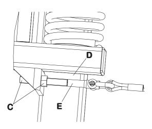
As a guideline for adjustment, follow the distance shown at the bolt assembly below:
