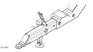
The support leg is stored in the bracket on the right side of the trailer when the sprayer is attached to the tractor. To remove the support leg: Lift the leg, remove the linch pin and pull out the support leg.
