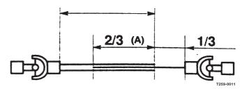
4. The two parts are shortened equally. Use a saw, and file the profiles afterwards to remove burrs.
