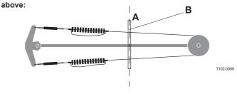
4. Suspend a weight of 4.5 kg from the straight edge-tocable contact point (B) and check deflection by measuring the distance from the straightedge to the cable. Cable should deflect 13-22 mm.
