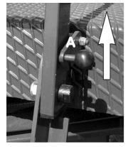
**Down:** Pull the handle (**A**) to disengage the locking device and tilt ladder down.
