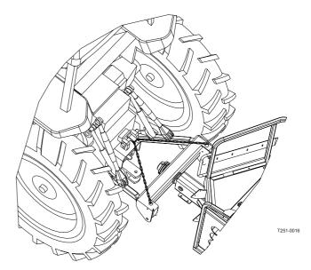
**NOTE!** If possible, lock the tractor hydraulic lever when the lift arms are in the correct position to avoid the sprayer weight resting on the stabiliser chains.
