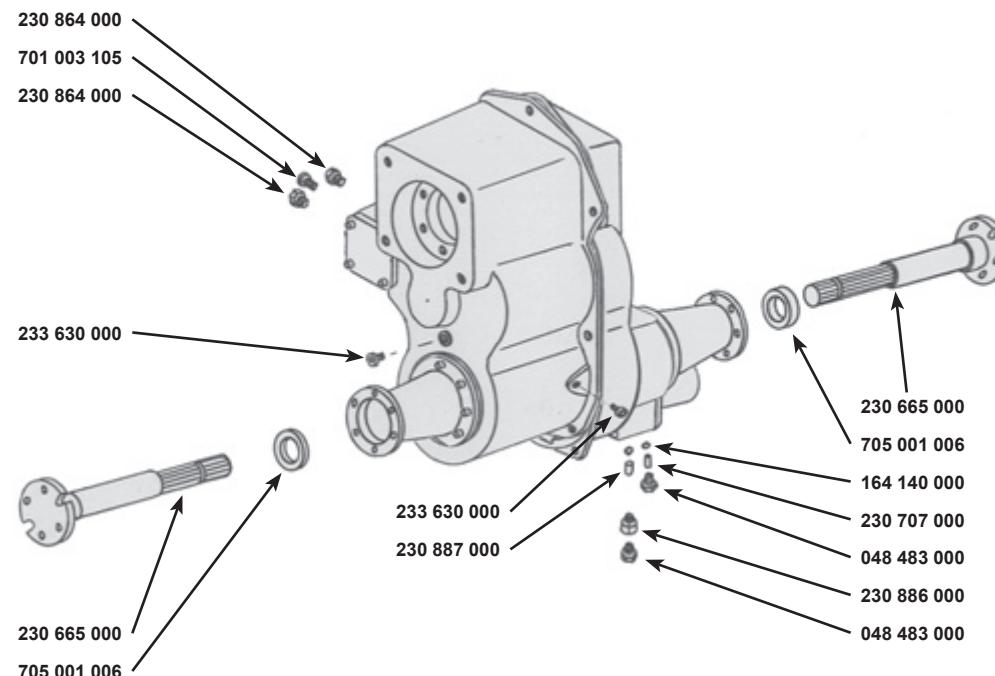
BOITE EQUIPÉE 25 KM/H AVEC 1 MOTEUR
