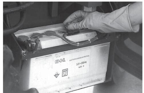
**Warning:** Do not smoke or use open fire when working with batteries. Explosive gases can be generated from batteries and cause serious injuries from fire or acid.
