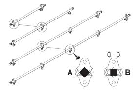
Nozzle tubes are supplied with one lock nozzle saddle per tube. A. The rest can slide lengthwise. B allowing for extension and contraction. Placement of nozzle tubes, connecting hoses and feed hoses. REMEMBER: Lubricate O-rings before fitting.
