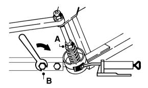
Lubricate coupling before adjusting spring tension. Slacken screw nut **A** to decrease breakaway resistance. Do not overtighten; better to loose than over-tight. Again minor adjustments in the field may be necessary.
