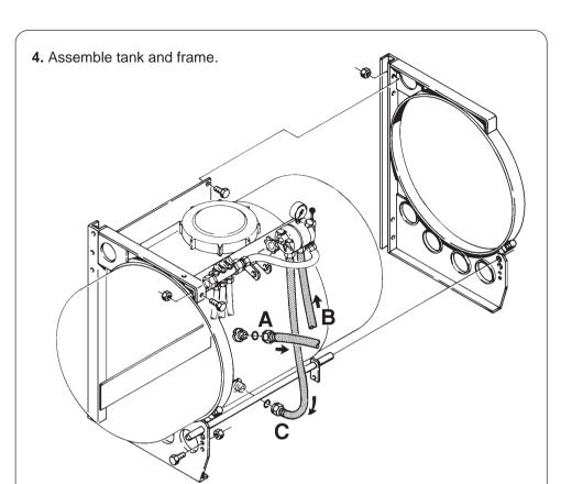
**5.** Fit hoses. Remember to lubricate O-rings before fitting.
