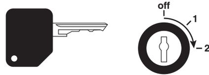
If the engine is cold, the engine preheat symbol will appear in the display. Leave the ignition key in position (1) until the symbol disappears before proceeding.
