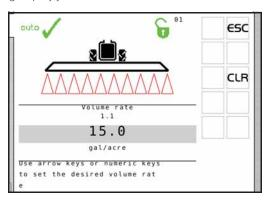
2. Adjust specific gravity when changing between a normal spray job and fertilizer spraying.
