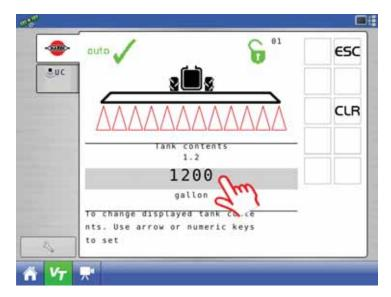
Enter the new tank contents value on the numeric key pad and select check mark to confirm.
