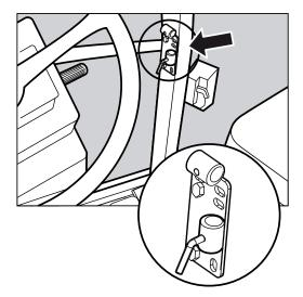
The supplied tractor pillar bracket (A) has a hole spacing of 3.9 in. (100 mm) and 4.7 in. (120 mm) and will fit most tractors. Threaded mounting holes may be hidden behind front corner cover.
