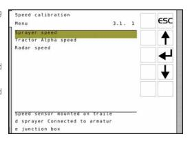
It is possible to calibrate the speed sensor in different ways. You may enter a theoretical speed constant or perform a practical calibration.
