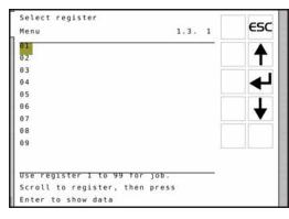
**5.** For SafeTrack, the sensitivity of the tractor hydraulic must be calibrated. Follow the instructions written in the bottom of the display.
