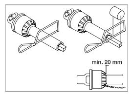
7. Fit the chains to prevent the protection guards from rotating with the shaft.
