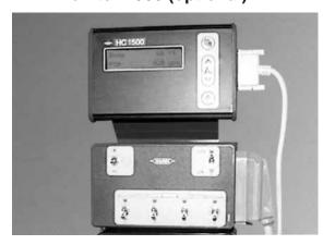
The HARDI® Monitor 1500 monitors the application rate. When used with the electric control unit switch box, correct area covered and up to 8 spray boom section control is possible.
