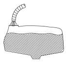
IF THE HOSE IS LEAD TO THE BOTTOM OF THE TANK, AND THE WATER PUMP AT THE WATER SUPPLY PLANT STOPS, CHEMICALS CAN BE SIPHONED BACK AND CONTAMINATE THE WATER SUPPLY LINES.
