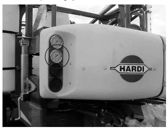
Boom Pressure and Manifold Pressure Gauges
