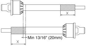
**Note:** The minimum allowable overlap for the shaft depends on the pump model.
