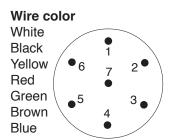
The wiring is in accordance with ANSI/ASAE S279.11.
