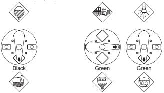
12. When the spray liquid is well mixed, turn handle on the Pressure Manifold towards "Spraying" position. Keep P.T.O. engaged so the spray liquid is continuously agitated until it has been sprayed on the crop.
