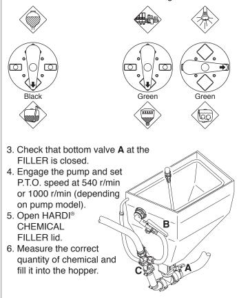
**Note:** The measuring scale in the hopper can only be used if the sprayer is parked on level ground! It is recommended to use a measuring jug for best accuracy.
