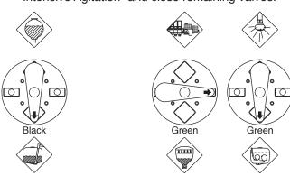
When the spray liquid is well mixed, turn handle on the Pressure Manifold towards "Spraying" position. Keep P.T.O. engaged so the spray liquid is continuously agitated until it has been sprayed on the crop.
