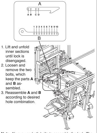
**Note:** Always use both bolts to assemble the lock. The setting must be identical on both sides.
