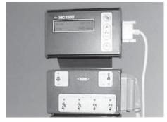
The HARDI<sup>®</sup> Monitor 1500 monitors the application rate. When used with the electric control unit switch box, correct area covered and up to 8 spray boom section control is possible.
