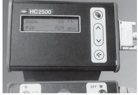
The HARDI<sup>®</sup> Controller 2500 permits automatic control of the application rate. This allows you to concentrate on driving as the rate is automatically maintained by the HC 2500. Press the "up" or "down" arrow keys to change the application rate. Easy, quick and simple. Up to 8 spray boom section control is possible.
