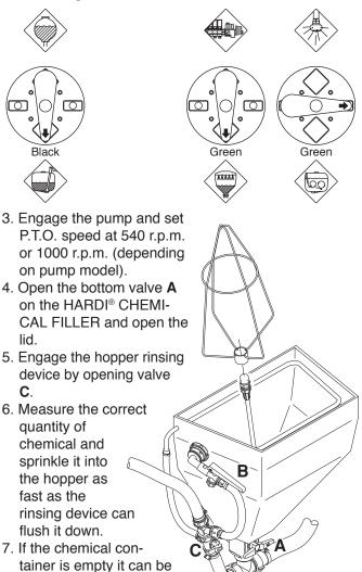
Bottle Rinse (optional). Fit the bag bracket and place the powder bag over the multi-hole nozzle and press the lever **B**.
