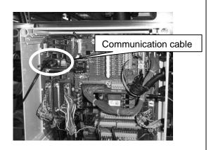
When the JobCom and PC is connected the PC can be powered up and afterwards the JobCom.
