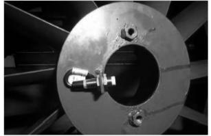
Picture 6 Fan speed sensor
