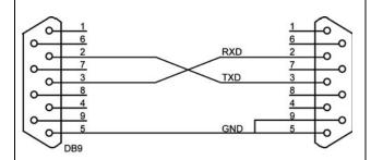
The cable is marked with "Hardware halt" at the end with the loop. The mark is on the cable or with a yellow sticker on the connector.
