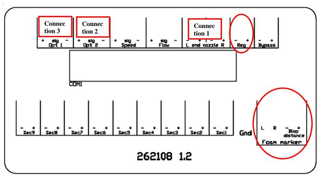
Picture 14 PCB for sections valves (9 section's PCB)
