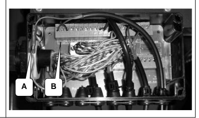
The cable from the Spray box has two lose wires which are not connected in the JobCom. These much be attached to the plug as shown on Picture 7
