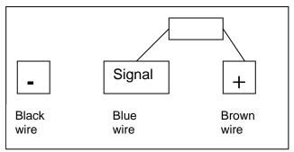
Figure 2 Mounting of the 10 K ohm resistance in the Jobcom
