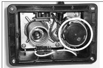
Pressure regulation valve knob is colour-coded Yellow.
