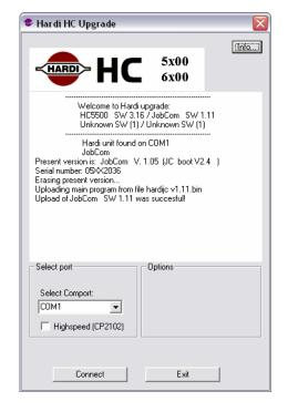
Reset Jobcom with HC5500 With new software in the Jobcom, it is necessary to perform a reset. To reset Jobcom with a HC5500 enter menu E.9.5. The PIN code is 74650.
