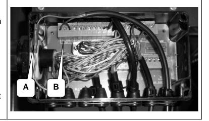
The cable from the Spray box has two lose wires which are not connected in the Jobcom.
