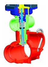
Picture 12 EFC without the equalization
