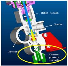
Picture 11 EVC with the equalization system
