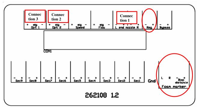
Picture 16 PCB for sections valves (9 section's PCB)
