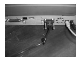
The communication cable is plugged into the Jobcom before it is switched on. The plug that is attached to the Jobcom is the one with the "Hardware halt" (yellow sticker).
