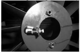
Picture 7 Fan speed sensor
