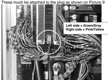
Picture 9 Connection of the two wires from Spray box cable
