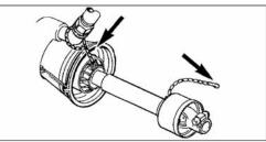
8. To ensure long life of the transmission shaft, try to avoid working angles greater than 15°.
