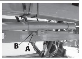
ATTENTION! The adjustment screw (B) must be open at least 1/4 turn or seal damage will occur.
