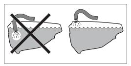
WARNING! Do not let the filling hose enter the tank. Keep it outside the tank, pointing towards the filling hole. If the hose is lowered into the tank and the water pressure drops at the water supply, chemicals may be siphoned back and contaminate the water supply lines and source.
