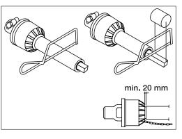
**7.** Fit the chains to prevent the protection guards from rotating with the shaft.
