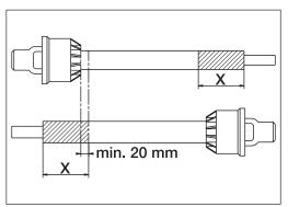
WARNING! The shaft must always have a minimum overlap of 2/3 the length.
