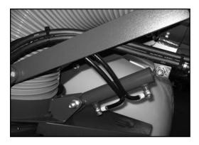
For a 180° rotation, another double acting outlet is necessary. This movement enables you to carry out the treatment on one side or the other of the CANNON, regardless of the direction the tractor is going.
