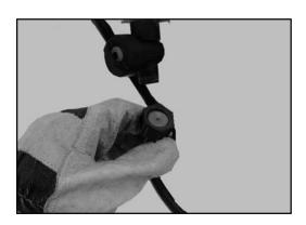
The CANNON model has a spout made of polyester and is only fitted on a pneumatic system. It includes 4 bi-jet holders with two nozzles each. Also included are three adjustable nozzles outside the spout which allow for proper treating of nearby crops.
