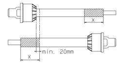
**Note:** The shaft must always have a minimum overlap 150 mm.
