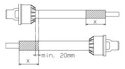
**NOTE:** The telescoping profiles must overlap at least by 1/3 of their length while in use.
