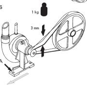
Tighten all counter nuts and replace guards after adjustment.
