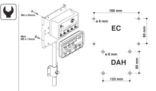
1. Mount the boxes on the holder delivered or a suitable bracket for the purpose.
