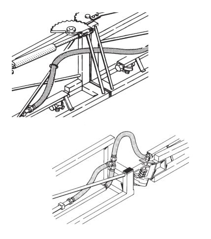
5. Secure feed and connecting hoses with plastic straps (approx. every 30 cm). Check that the hoses do not catch or pinch during **folding and unfolding.**
