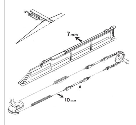
6. Midway on the wire of the inner section, check the tension. A 10 kg force the wire should move a maximum of **3 mm**. Adjust rigging screw if necessary.
