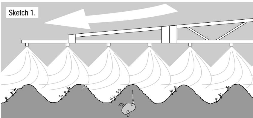
**Sketch 1.** The “Ridge effect”, which allows weeds on the lee side to be not contacted by the herbicide, when spraying conventionally under windy condition.
