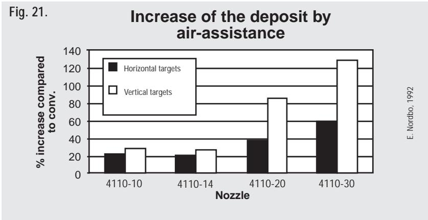
**Fig. 21.** Testing in a laboratory shows that the magnitude of deposit increases on artificial and horizontal targets when air assistance is applied. The horizontal targets are simulating broadleaf weeds or crops, the vertical grass weeds or stems or ears on plants. For all relevant nozzle sizes at least 20 % increase in deposit has been observed.
