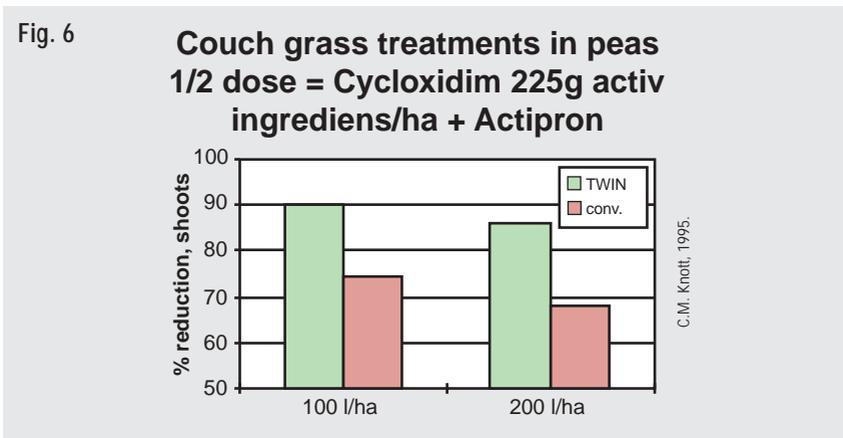
**Fig. 6.** Control of couch grass - a perennial rhizotamous grass weed. Air assisted spraying gave a considerable better control of this serious grass weed than conventional applications at both 100 and 200 l/ha. The results are at the recommended dose and show a tendency of higher biological activity at the lowest water quantity.
