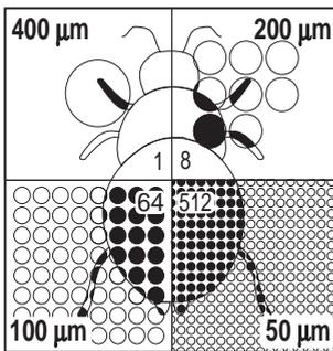
**Fig. 3.** Each square represents equal water quantities but atomised into four different droplet sizes. The smaller the droplet size - the better the coverage. The volume rate can be reduced significantly - generally by 50 % of conventional use, sometimes more, because the small droplets are much more efficient for coverage - and with the TWIN air assistance they are safe to use.
