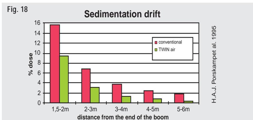
**Fig. 18.** “Dosing” on the downwind out of the treated area. TWIN has halved the deposit out of the target area, compared to spraying with a conventional sprayer. Both systems applied 150 l/ha of Fine Sprays (4110-12, 3 bar).
