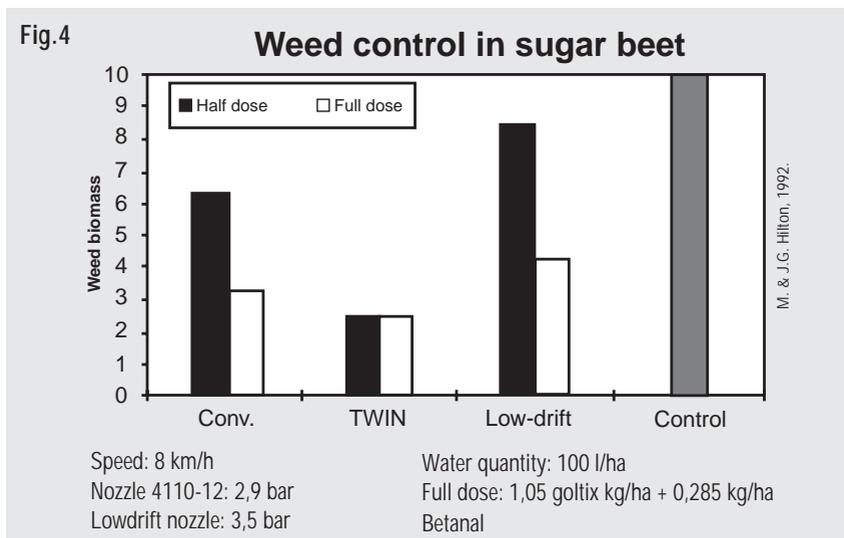
**Fig. 4.** The weed biomass was evaluated on a scale from 0 - 10, where 0 means 100 % kill and 10 is no effect. For conventional and Low-drift nozzle full dose was more efficient than  $\frac{1}{2}$  dose - TWIN maintained the good control also with  $\frac{1}{2}$ -chemical dose rate.
