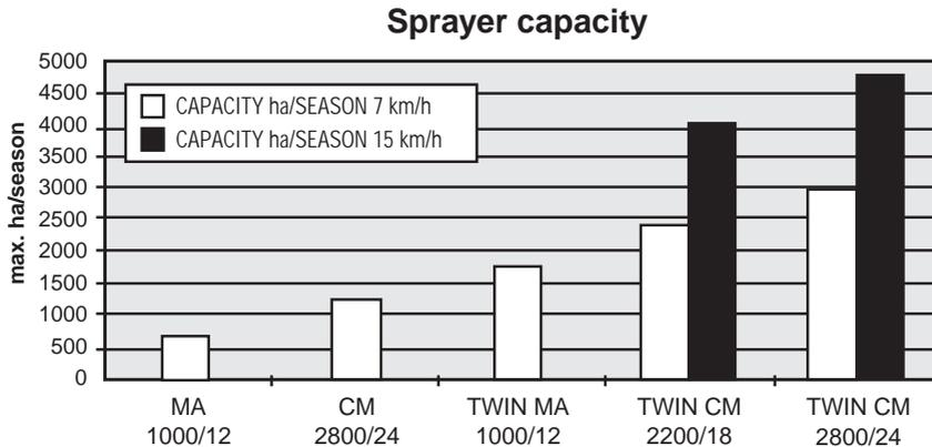
**Fig. 1** Theoretical capacity ha/season. The figure reflects partly that spraying with TWIN is seldom limited by the wind and furthermore the increased work rate due to lower water quantity with TWIN. The effect of higher driving speed is shown in separate columns.
