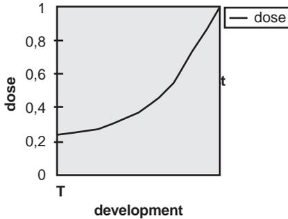
**Principle sketch** For example, when spraying herbicides in beet or potatoes it is generally accepted that approx. 2 days are available to spray the area when the weed is at the dicot stage and the lowest possible dose can be safely used.
