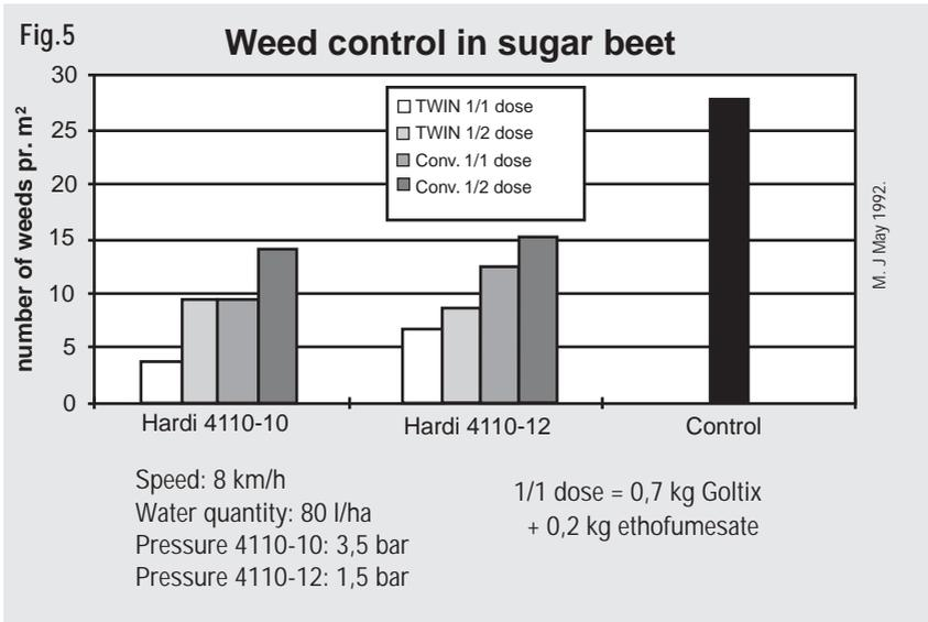
**Fig. 5.** Air assisted spraying at full dose gives the highest weed kill. TWIN at half dose rate is as efficient at conventional spraying at full dose.
